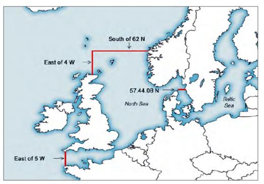
Fig. 1. Borders of *sulphur* emission control areas SECA [4]
